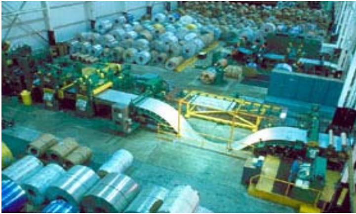
RyersonTull: Precision levelling of aluminium and steel
