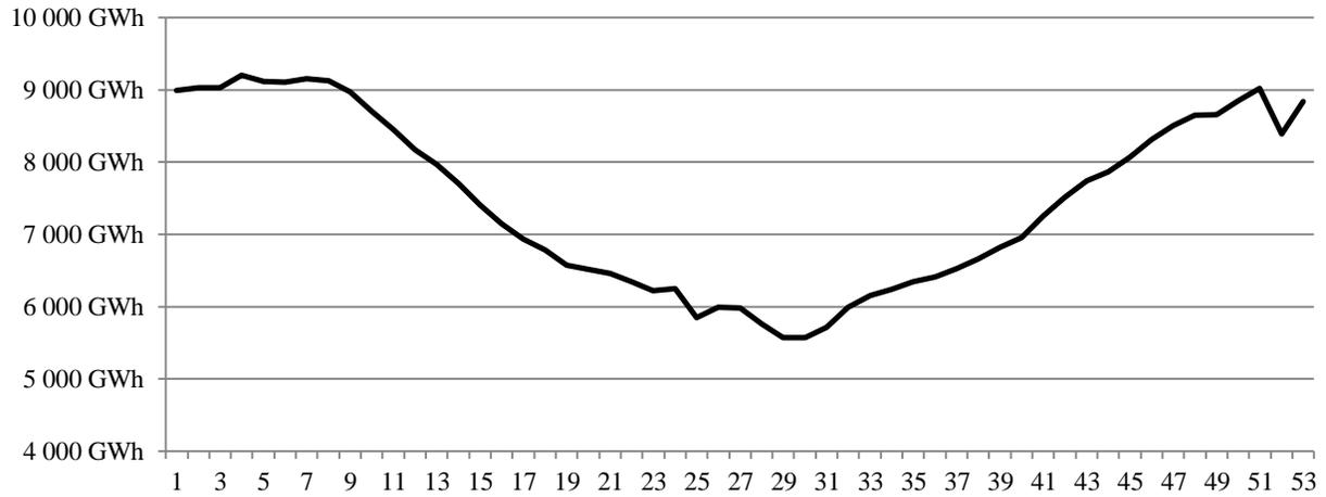
When comparing the average weekly electricity demand in Figure 6 and the temperature curve in Figure 7 below, it can easily be seen that electricity demand seems to be inversely correlated with temperature: the demand is at its peaks during the coldest weeks of the year, whereas the warmest weeks of the year are accompanied with the lowest power demand levels in the annual cycle.
