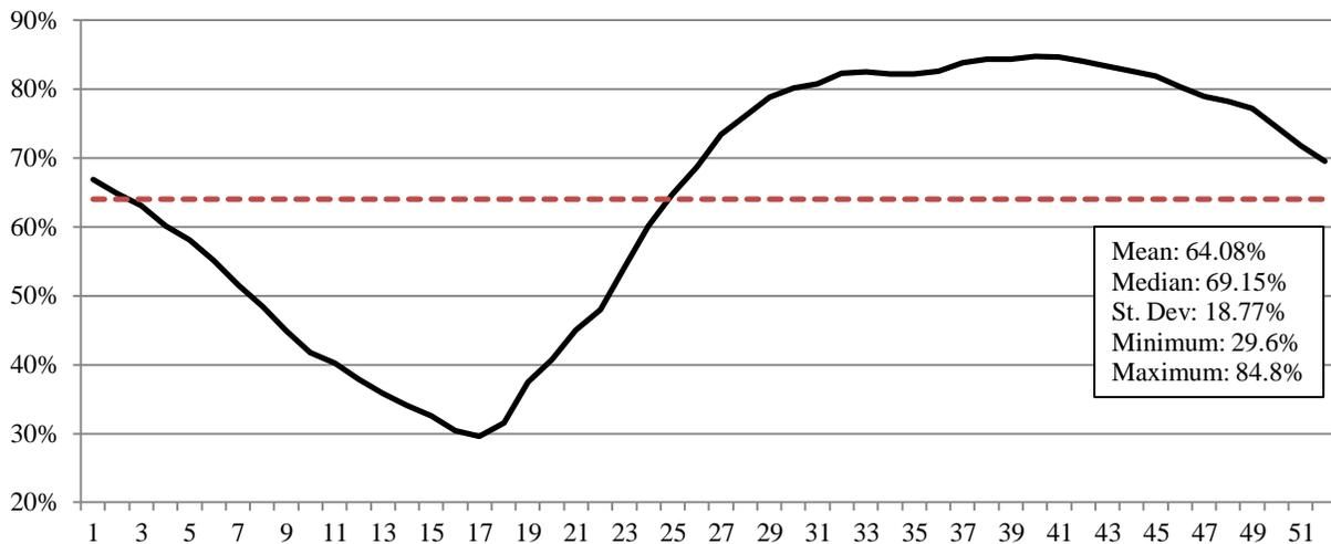
As shown in the Figure 10, the water reservoirs reach their lowest levels – ca. 30% of the maximum capacity – in the spring around weeks 16 and 17, after which the precipitation and melting snow begin to fill the reservoirs again and the reservoir levels increase steadily until reaching their maximum filling levels of ca. 85% around weeks 40 and 41 in the autumn.
